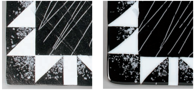
Figure 5 The design on the left was fired face down, The design on the right was fired face up. Notice the crisp edges of the design on the left.
