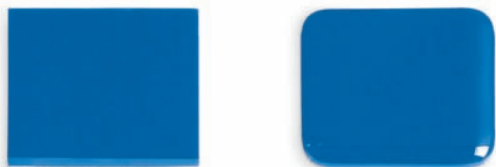
Figure 1: Two, 1/8" (3mm) layers fired to 1500°F (816°C). Notice that the area covered stays the same and the edges are straight.
